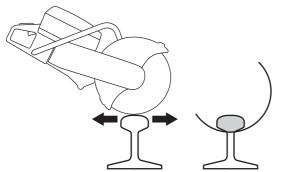
• When you have cut through the head (A), you continue cutting the rib (B) and foot (C).
