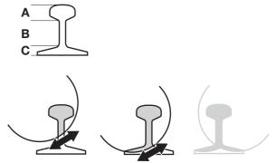
If the cut cannot be completed from one side, the power cutter must be turned around.
