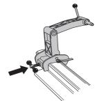
Mount the power cutter with its right side to the fixture.
