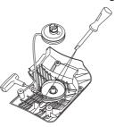
Remove the recoil spring by turning the starter over and loosen the hooks, with the help of a screwdriver. The hooks hold the return spring assembly on the starter.
